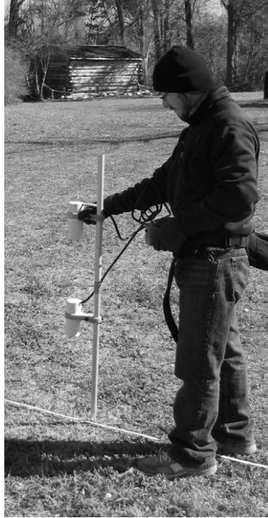
Figure 3.10 The Geometrics G-858 cesium vapor magnetometer shown being used in gradiometer mode.
