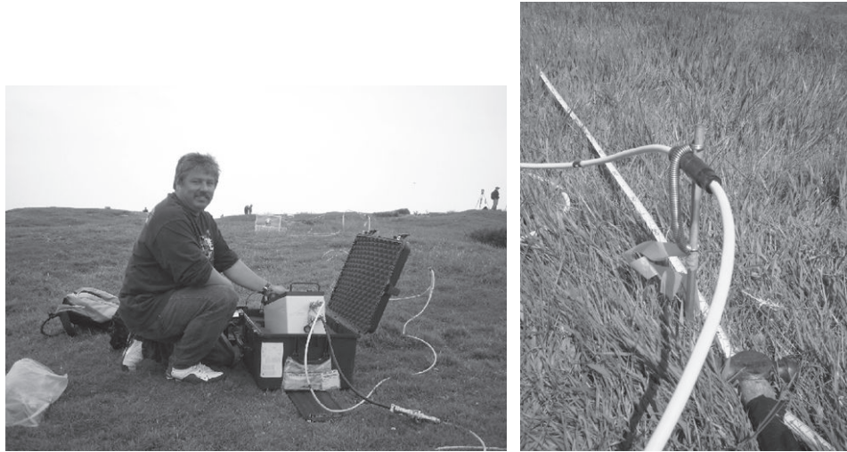
Figure 4.16 (Left) Multi-electrode resistivity system from AGI Geosciences, Inc.; (right) close-up of an electrode installation.
